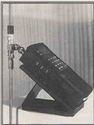
The dipole fitted to an airband scanner.
