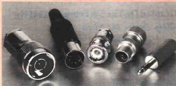
Left to right: N-type, 5-pin DIN, BNC, Belling-Lee coaxial and 3.5mm jack.
