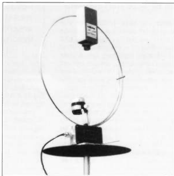
Fig. 12.6: Lower and medium h.f. and h.f. loop antenna with tunable inductance inside a split screen; note that loop inductance may contain several turns of insulated wire depending on diameter and frequency of operation.
