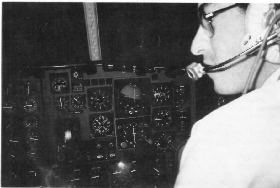
Godfrey steers a left turn in a Lockheed C-130 Hercules Mk 1 simulator. Altitude 1750 feet, airspeed 179 knots, heading 100°, using 25° of bank with gear and flaps up. (Photo: Christine Mlynek.)
