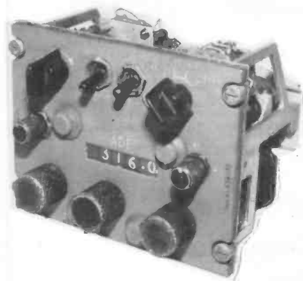
Fig. 2.1: Typical a.d.f. radio controller.
