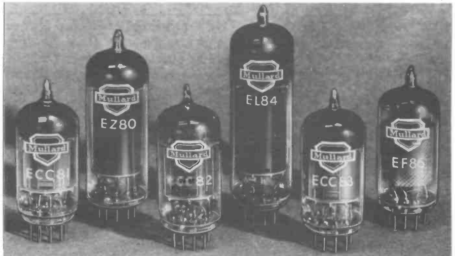
Mullard valves for audio amplifiers. EF86, ECC81, ECC84, EL84 and EZ80.
