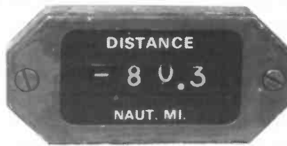
Fig. 2.6: Typical d.m.e. display.
