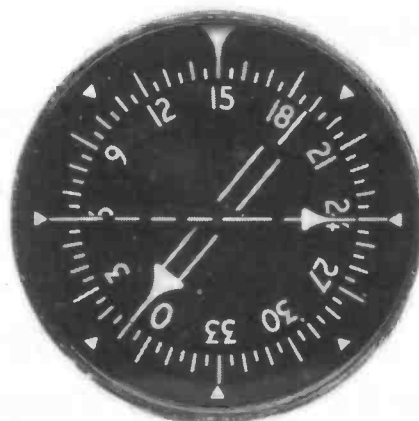
Fig. 2.2: Typical radio magnetic indicator.
