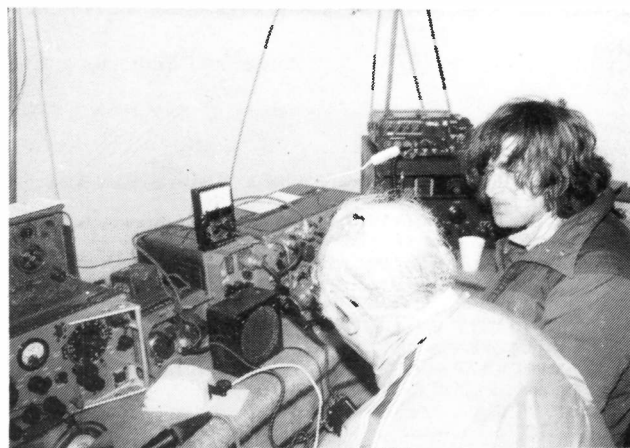
Reigate Amateur Transmitting Society joined in the recent 'VE' Day commemorations by operating a station under canvas on the coast at Littlehampton, Sussex. Seen here is an Army 62 Set in operation, with a U.S. Patrol Fone resting on an AR88 receiver; Ron Brown, G3JRC, and David Skilton, G1KPU, are in position. photo: Phil Pardey
