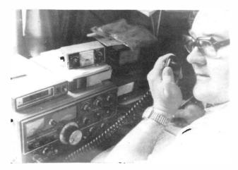
The station of Bob Owen, G4IJG, a well-known member of Stockport Radio Society. Licenced in 1979, Bob runs a Trio TS-520S into a 3-element beam with an 18-AVQ as backup, and this combination has brought him plenty of DX. A beam rotator indicator can be seen to the lower right of the TS-520S.
