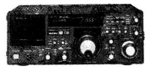
THE LATEST SOMMERKAMP — FRG7700 COMMUNICATION RECEIVER. 150KHz - 30MHz multimode, digital frequency readout, 12 programmable memories, variable bandwidth, built-in clock/timer. Price £389.00.
