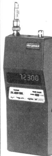
IM-2400 Hand-held Frequency Counter Measures 50Hz to 512MHz in two ranges. 7 digit LED Display. Crystal-controlled 10MHz time base. Operates on nickel-cadmium batteries or line current with optional eliminator charger. Swivelling Telescopic Antenna optional.
