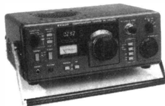
Trio R1000 PLL C&L SWL Communications Receiver 200kHz to 30MHz. £285.00
