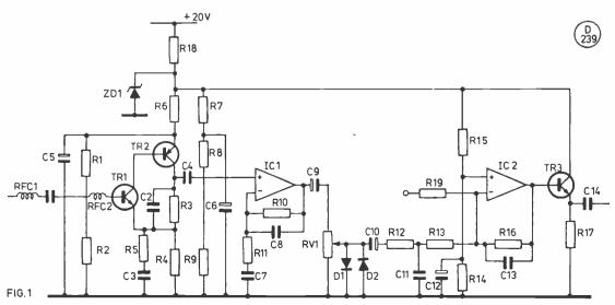
caused to roll-off at low frequencies by C3, and at high frequencies by C2. The RF chokes have been included to prevent any RF feedback that may occur, especially if the aerial is fairly near the microphone; they consist of three turns of enamelled wire on a ferrite bead. The supply for this stage is well smoothed by R6 and C5 because any ripple on the supply line at this stage will be amplified through the whole system and be quite significant at the output.
