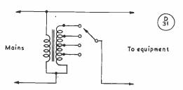
Note: Secondary must be capable of carrying fullmains current required by the equipment.
