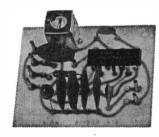
455 kHz FM Discriminator Amplifler. Limiting threshold 100uV. Amplitude modula-tion rejection 40dB. Audio output voltage at 1 kHz 200-300mV frequency deviation + or — 3 kHz. Price £5.00
