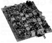
AT 122. A complete transmitter exciter unit for 144–145 MHz on AM or FM. VFO controlled or fixed channel operation. Complete with microphone pre-amp, speech processor including active audio filter. I watt output. FM. 25 watt AM. Output impedance 50–75 ohm adjustable. Frequency deviation 3–10 kHz adjustable.
