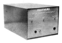
This unit will power your mobile rig or any other equipment including charging batteries. It is short circuit proof and protected against thermal overload. Substantial RF filtering is provided and the output voltage is adjustable over the range 11 to 14.5v.
