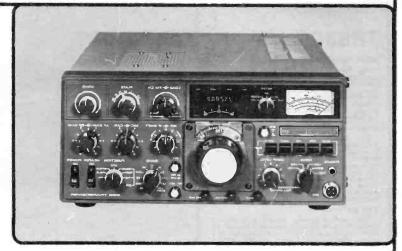
SIDEBAND SUPPRESSION: Better than 50dB. SPURIOUS RADIATION: Greater than 60dB (Harmonics more than 40dB) RECEIVER SENSITIVITY: Better than 0.25 $\mu$ V. RECEIVER SELECTIVITY:
