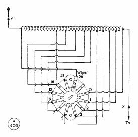
Circuit of the end-fed Aerial Loader Unit, as described in the article by G3OGR. Essentially, what it does is to provide the required inductance to bring almost any short aerial to resonance on almost any band—obviously, there are extremes which the Loader could not accommodate.
