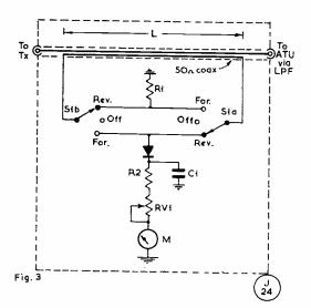
Fig. 3. Monimatch modification to enable the diode to be switched out in the "off" position—see text. Values are: C1, .001  $\mu$ F; R1, 33 ohms; R2, IK; RV1, 5K pot.; L, pick-up wire less than 1/20th wavelength.
