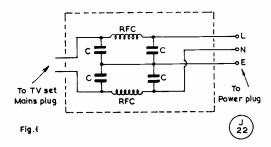
Fig. 1. A mains filter suitable for installation in the input lead to a TV receiver. The chokes can be Electroniques Type CCC-2, and the condensers .01  $\mu$ F, rated 1000v. working.
