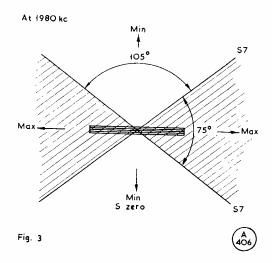
Fig. 3. Directivity pattern obtained with the Frame Aerial on transmission.
