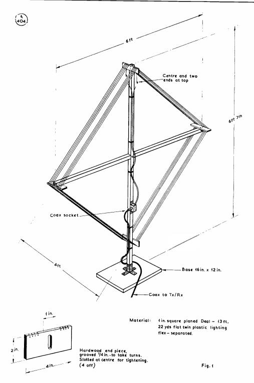
Fig. 1. General constructional detail, Frame Transmitting and Receiving Aerial for Top Band.
