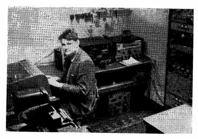
Very recently licensed is James Heck, G3WGM, of Homefield, Hartsbourne Avenue, Bushey Heath, Herts., whose main interest at present is 80-metre AM/CW, and RTTY. He runs a 60-watt Tx with an end-fed aerial, and his Rx is a BRT-400. The machinery for RTTY consists of a Creed 7B teleprinter, with a tape auto-transmitter, all of which has been in operation for some time under SWL conditions.
