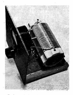
Simple enough—the Loader Unit described by G3OGR can be used to operate almost any length of end-fed aerial on any band, within reasonable limits. There are some extremes that cannot be covered—something very long for 10 metres or exceptionally short for Top Band, for instance.
