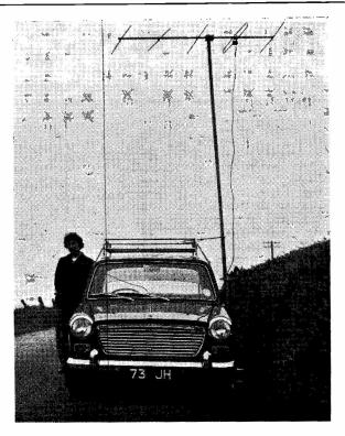
The GM5UM/P set-up for two-metre operation during his recent safari. The aerial mast is a tight fit through a hole in a flat dural plate clamped to the roof-rack by wing nuts, and the butt end of the mast goes through the central hole of one of those large wooden reels on which wire is wound; this makes a firm base, and the beam is easily turned. During the trip, May 29 to June 9, 23 contacts were made on 145.8 mc, from Argyll and Wigtown shires, running 9w. on GW and 7 watts on telephony.
