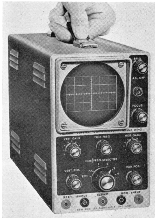
Though the new Heathkit Model OS-2 Oscilloscope is small and compact, it has a very complete specification, and is suitable for general servicing and home workshop applications. The tube is a 3in. medium persistence, showing a green trace, and features include a broadband Y-amplifier, external horizontal input and synchronisation by an automatic lock-in circuit. As is usual with all the excellent range of Heathkit apparatus, the OS-2 is available either factory-built or in kit form.
