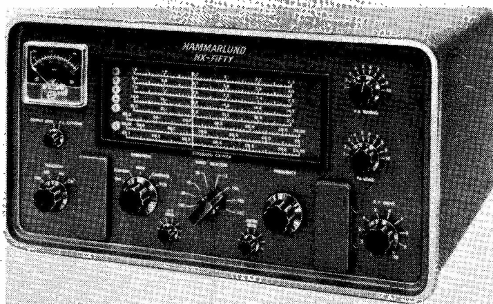
General external appearance of the HX-50 Transmitter/Exciter, manufactured by Hammarlund and handled in this country by K.W. Electronics, Ltd. It gives CW/SSB output on all bands 10-80 metres, a modification kit being available for 160 metres, and is a very attractive piece of equipment, easy to handle and operate. It is reported on in detail in the article herewith.
