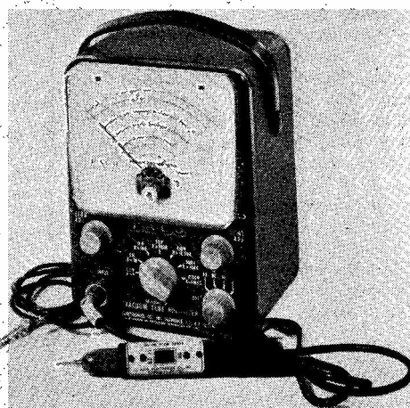
The new PACO V.70 Valve Voltmeter employs a balanced bridge circuit for maximum sensitivity and stability. This instrument has seven DC and AC ranges covering up to 1500v.; a range of 0-4000v. peak-to-peak; an ohmmeter coverage of 0-1000 megohms; and can make decibel measurements between -6 dB and +66 dB. It is £22 12s. nett, and is available in kit form at £20 8s.
