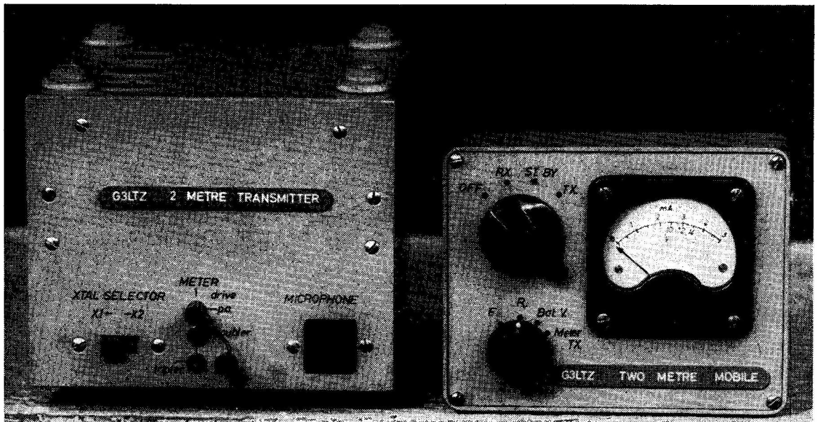
General view of the G3LTZ transmitter in its case (left), with the control unit, constructed as a separate item — see text and Fig. 3. The PA is a double-tetrode, and some constructional details behind the panel and under the chassis are shown in the other photographs.
