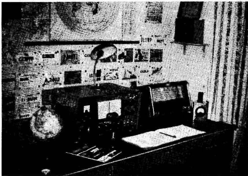
Typical medium-power amateur station using commercial equipment—a K.W. Vanguard transmitter; Eddystone 888A receiver, on tilt blocks; and an Acos microphone. At right is an absorption wavemeter, and behind the globe a monitor unit. On the wall is our DX Zone Map, and beside the Webb's log-book is a copy of the latest (when this photograph was taken) issue of "Short Wave Magazine." By the way, whose station is it—we haven't a clue!
