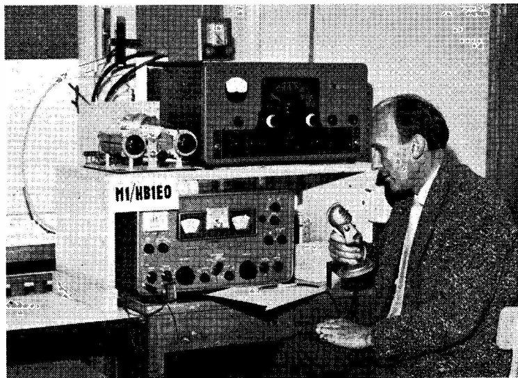
When HB9EO was in San Marino during November 1-10, he was signing M1/HB1E0 and in 8 days' operating made some 1,500 contacts, of which 170 were with U.K. stations and about 40 with VK/ZL. His transmitter was a Viking Valiant running 200w., the receiver a Hammarlund HQ-180, and the aerials a trap dipole and 20m. doublet.
