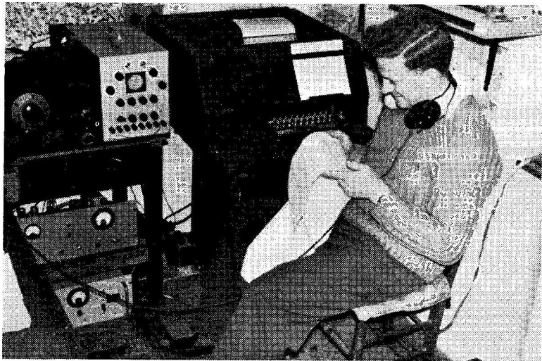
G3GNR, Amersham, who is active on RTTY, has the G3BST FSK converter — described in our March-April, 1960, issues — and a page printer, shown to the right on the bench. There is now a small but active group of G's running radio teleprinter as a regular means of communication on the HF bands.
