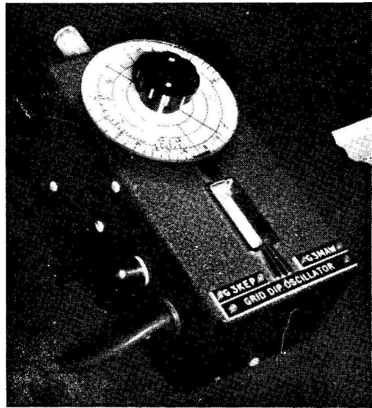
General view of the Grid Dip Oscillator described in the article. The dial is calibrated for the ranges covered, and the coil in use plugs in at the top of the box. The magic-eye looks out from beneath the dial.
