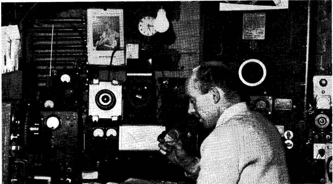
G3JHK, Stockport, Cheshire runs a home-built all-band transmitter incorporating a Gelson VFO driving a pair of 807's in parallel; these are plate-and-screen modulated by a pair of 807's in Class-B zero bias. The PA input is 140 watts, phone mainly, on 10 and 15 metres. The receiver is an HRO, and the aerial is a home-built tri-band beam, at a height of about 30 ft.
