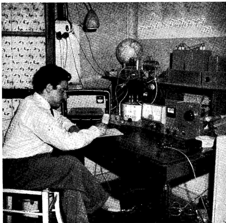
When G3AMM was on his way to Spain during the summer he met F2IG, Toulouse, who runs a Geloso VFO-PA 807 transmitter, with various aeriels, the receiver being an amateur-band converter working into an ordinary BC set.
