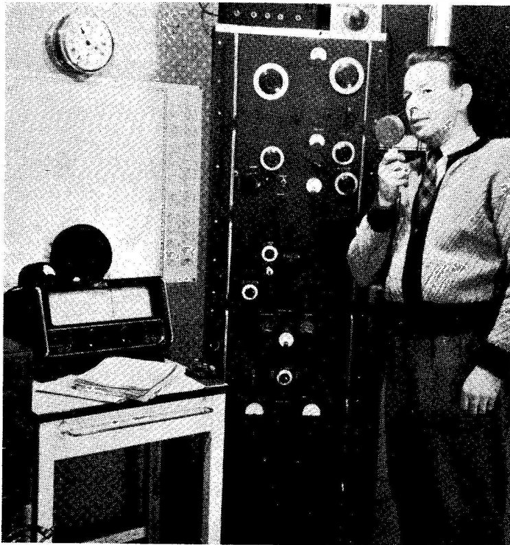
G3KPM, Holloway, London, was licensed in October 1955, after a long apprenticeship as an SWL — always the best way of breaking into Amateur Radio. Except for the Eddystone 750 receiver, the station is entirely home-built; the transmitter is in six pull-out racks in an aluminium cabinet, and total screening is achieved. The PA is an 813 running the full 150w. on the 10-80 metre bands, with a separate self-contained 10w. transmitter for Top Band. Modulation on the 813 PA is by a pair of G.E.C. KT88's in Class-AB2, and for 160 metres an 807 is used. Auxiliary equipment includes a TVI indicator, aerial filter unit, absorption wavemeter and grid dip oscillator and, in the interests of safety, an overload relay to cut power to the whole outfit. The QSL policy is 100% on all first-contacts. G3KPM also works mobile on 160, 80 and 40m.
