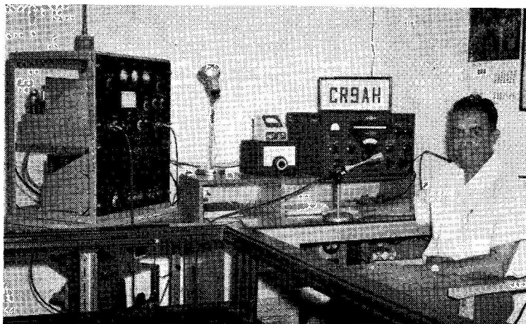
CR9AH, Macao, China, is on SSB with a pair of 6146's in Class-AB1 as a linear PA. His receiver is a Collins 75A-4.
