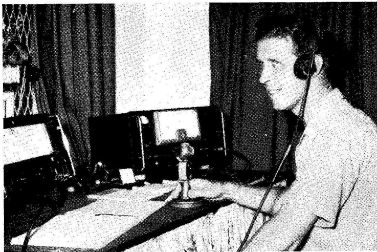
VS1FJ, Singapore, who is well known as G3IDC of the R.A.F. Amateur Radio Society, runs only 25 watts, but has worked 210 countries in 40 Zones, with 176C confirmed in 39Z. His aerial is an 86-ft. Zepp-fed top for the four HF bands, as well as a ground-plane for 20 metres. The key is a Marconi marine type, the modulator runs a pair of G.E.C. KT66's in push-pull to give about 12w. of audio, and the microphone is a Chinese copy of an American moving-coil type, made in Shanghai! The receiver at VS1FJ is an Eddystone 888.
