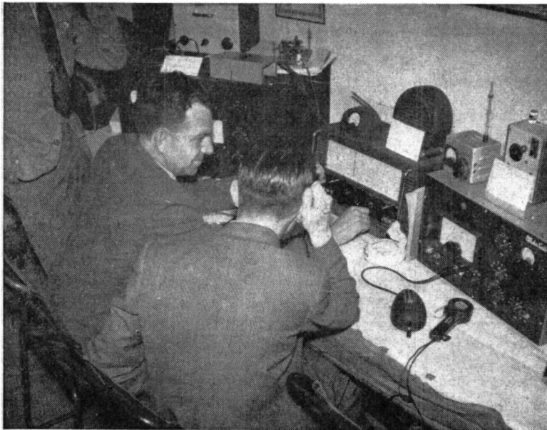
For the recent Model Engineering exhibition in Belfast, the City of Belfast Y.M.C.A. Radio Club set up G16YM/A. The bench equipment included an Eddystone 888 receiver, with Minimitter and Panda Cub transmitters. This photograph shows G12DZG operating, with G13MBB (back to camera). Using a sloping aerial about 200-ft. long, numerous contacts were made, all over the world.
