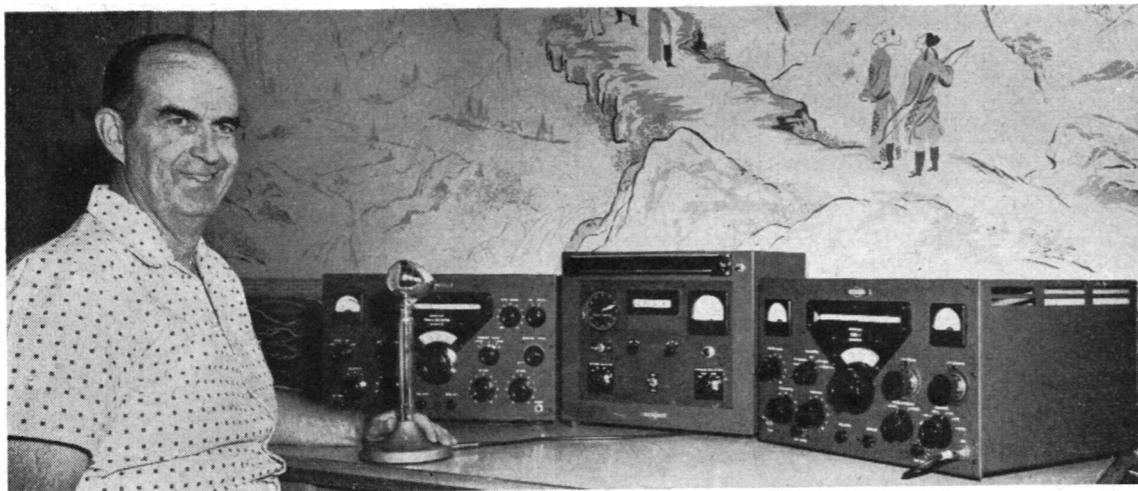
When W6ITH signs FS7RT and PJ2MC on his visits to the Island of Saint Marten (French and Dutch) he has a KWS-1 transmitter, SC-101 station control unit and 75A-4 receiver, all of Collins manufacture. The SC-101, centred in this photograph, contains speaker, aerial matching and switching controls, beam direction indicator — and a clock. Murals by the XYL.
