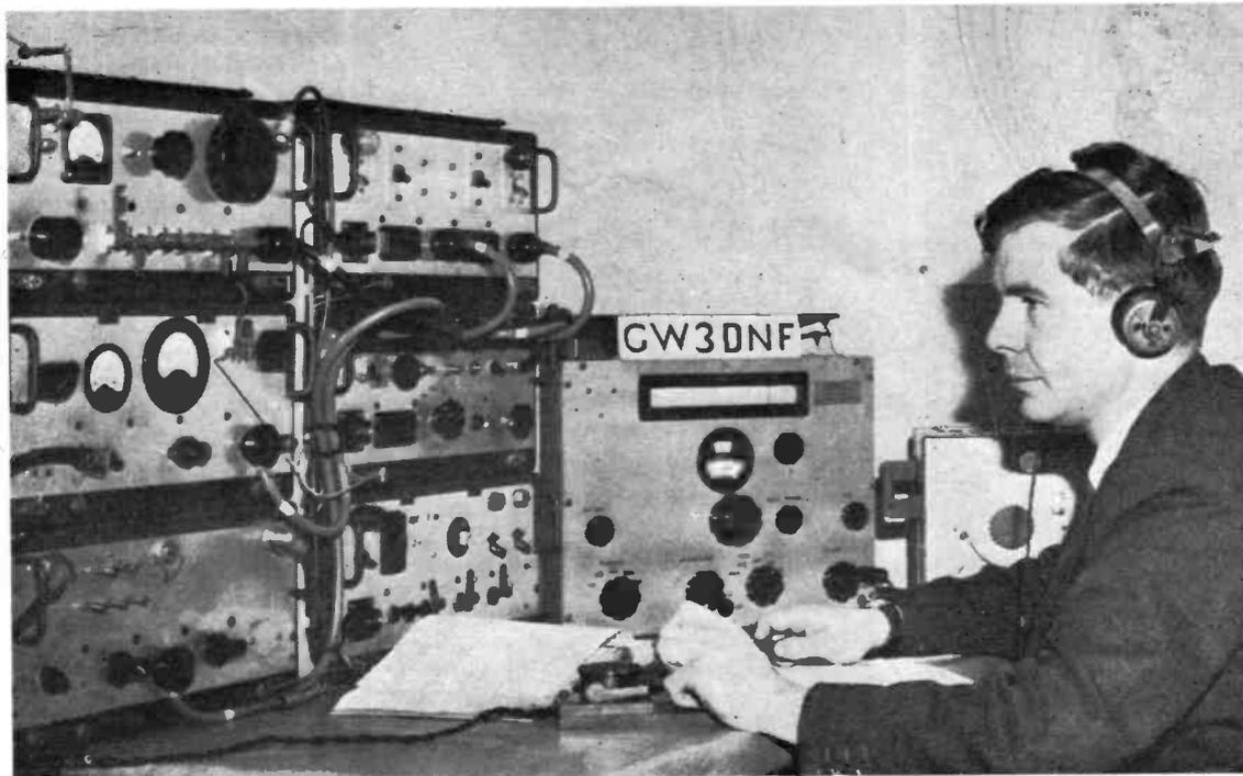
Station of GW3DNF, Chirk, Denbighs., who at one time was G3DNF in London. Though the gear looks elaborate and high-powered, in fact no more than a maximum of 12 watts is put in on all bands. The aerial at present in use, at a very good location, is a 200-ft. wire, end fed.
