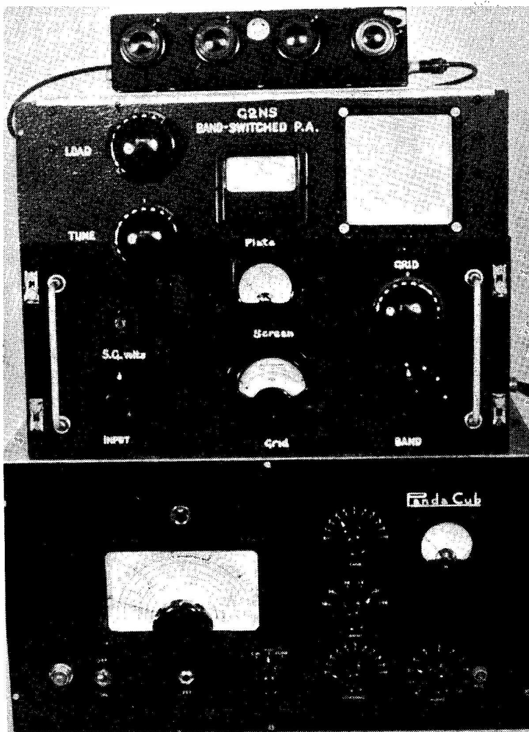
Front view of the 150-watt amplifier, discussed by G2NS, for which the drive unit (lower section) is a Panda Cub. Above the 813 band-switched PA, fully described in the text, is an aerial filter.
