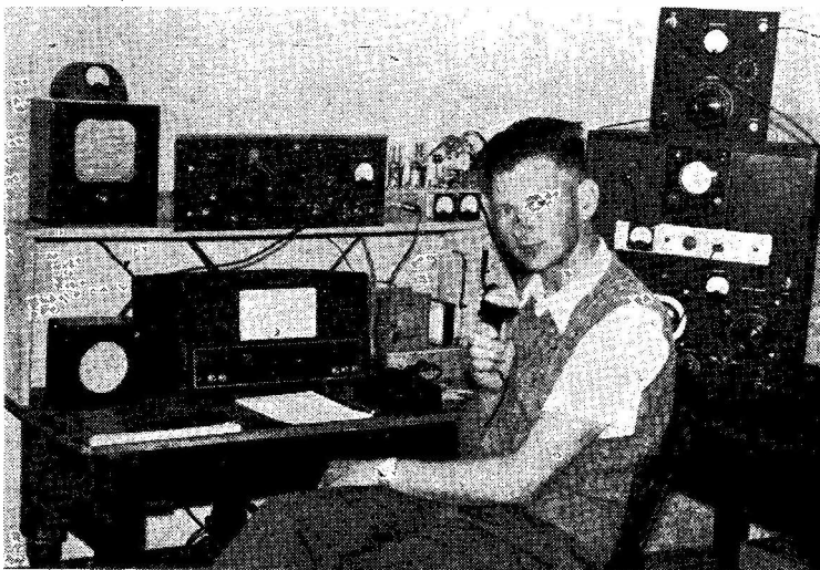
GW3INV is at Wrexham, Denbs., and has an S.640 as main receiver; the transmitter, lower right behind him, is on 80 metres, above which is its modulator, complete with oscilloscope. The aerial tuning panel is on top of the modulator and other equipment visible is for two metres. On Eighty, GW3INV uses an indoor 66-foot aerial.
