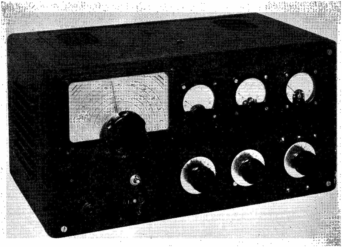
Front view of the 160-metre transmitter described in detail by G5JU in the accompanying article. The VFO control is the large dial and the three scaled knobs control condensers C15, C21, C22, which can be located in the other photographs. The PA output circuit is designed to load into an aerial of "random length"—that is to say, any type of aerial, within reason, can be resonated in the 160-metre band.
