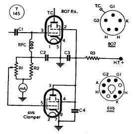
Fig. 1. A single 807 PA (top) with a 6V6 clamper valve which not only protects the PA (see text) but also, by means of R1, can be used to give smooth control of DC power input to the RF amplifier.
