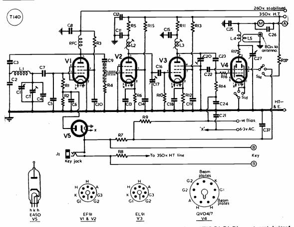
Fig. 1. RF section of the 160-metre transmitter described by G3FRV. It is a straightforward VFO-BA-BA-PA arrangement, designed for full break-in working and relay control on telephony. The VFO features the extremely stable Tesla oscillator circuit, and miniature valves are used throughout this section. The design for the modulator will be given next month.
