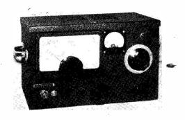
Front view of the RF-Modulator section of the 160-metre table-top transmitter described in the article
