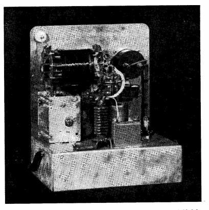
Rear view of the Beginner's Transmitter, showing the general arrangement behind the panel. The tuning inductance L is top left, mounted across C2 (left) and C1. The RF choke, with its sectionalised windings, can be seen mounted vertically beside the 807 oscillator valve, on the near edge of the chassis. The condenser to its immediate right is C6, with the crystal current indicator (a 60 mA flash-lamp bulb) mounted to the right
