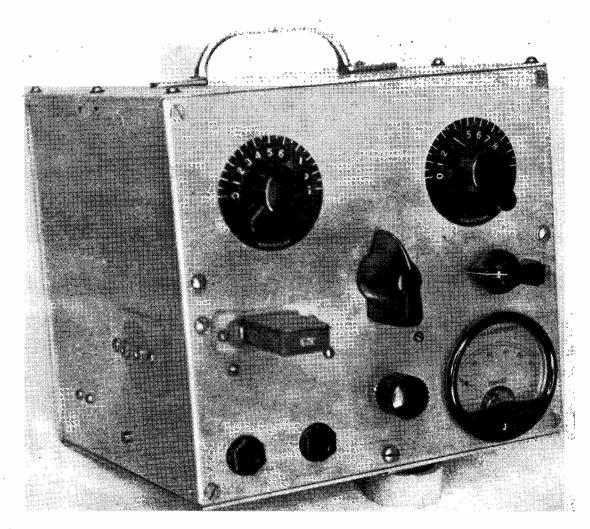
General appearance of the all-band CO-PA "Caravan Transmitter" designed by G2XX. Though approximate dimensions overall of his model are only 7 ins. by 6 ins., by 6 ins., the frequency coverage, band-switched, is 3.5 to 28 mc inclusive, either CW or phone. The Brimar 5763 PA takes up to 15 watts input and the total load on the car battery is about 7 amps. at 12 volts. Ap external dynamotor power supply is used.
