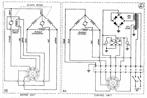
Fig. 1. Wiring layout of the Controller, showing inter-connection of the Autosyn transmitter (geared to the drive motor) and the indicating Autosyn unit.
