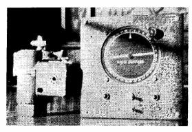
In this view, the Autosyn motor unit is to the left of the Controller
