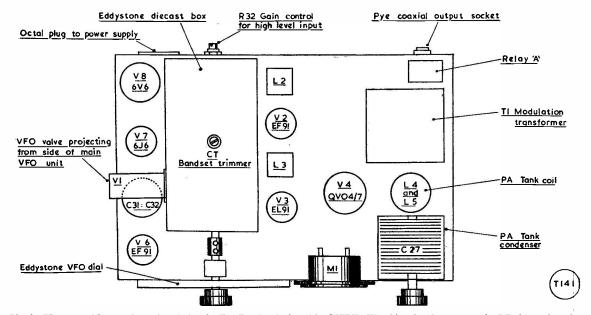
Fig. 2. The general layout above chassis for the Top Bander designed by G3FRV. His object has been to get the RF side and modulator into one cabinet, the power pack being a separate unit. This transmitter could, of course, be built as three separate units.
