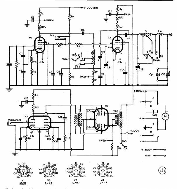
Circuit complete of the transportable band-switched CW/Phone transmitter designed and described by G2XX. VI, V2, is the RF section, using a 6CH6 at VI and a 5763 as PA; a pi-section tank circuit is used for matching any length of wire on any band. Modulation is by plate-and-screen control, the speech amplifier-modulator section being V3, V4, using miniature twin-triodes. A switched meter, with suitable shunts R6, is used for the various current measurements. All values are given in the table.
