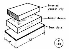
Fig. 2. Mechanical assembly of the portable transmitter/ receiver described by G8PG. The metal chassis is fixed to a base plate and the upper part of the chassis is enclosed by a wooden cover. When fitted together, the whole thing can be carried comfortably under one arm.
