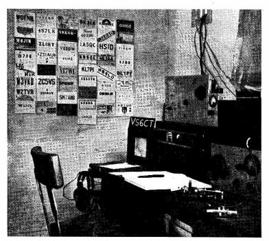
VS6CT is located at Little Sai Wan, Hong-Kong, and is actually the station of the local R.A.F. Amateur Radio Club, formed in November 1953. Original members were VS6DE (ex-G3HRY), VE5BO, G3KGM and G3KLP (when serving in VS6). The receiver is an AR88 and operation is on 40 and 20 metres running 25 watts in a VFO/BA/FD/PA layout, with a selection of aerials.
