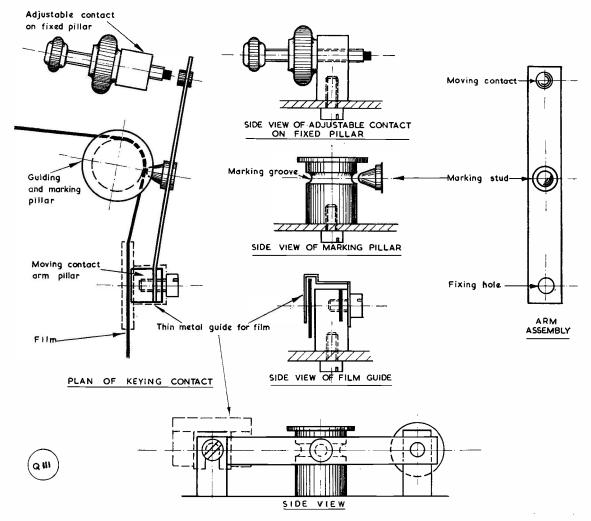
Fig. 2. Arrangement of the keying head, showing how the marking pillar is grooved and the tip of the marking stud rounded to give positive make-and-break at the keying contact; this groove, and the rounding of the marker stud, may be a matter for adjustment, the aim being to obtain sufficient "throw" on the keying arm with no tendency for the marker stud to catch in the tape perforations.
