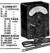
A conveniently compact 21-inch moving coil precision meter for making D.C. measurements of milliamps, volts and ohms. The total resistance of the meter is 100,000 ohms, and full scale deflection of 300 v. or 600 v. is obtained for a current consumption of 3mA: or 6mA. respectively
