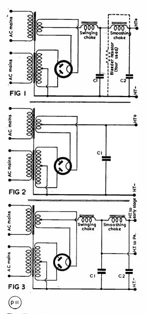
These diagrams incorporate the points made by G5JU in his article. Fig. 1 is the standard arrangement; in many applications, the smoothing choke can be dispensed with. In Fig. 2 is shown an acceptable arrangement when the anodes of modulator valves only are being supplied. Fig. 3 shows the circuit to use when it is impracticable to run two separate power supplies; this arrangement is preferable to allowing the whole load current to flow through a single arm.
