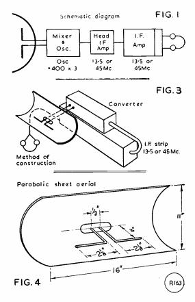
Showing the general layout of the 25-centimetre superhet converter designed by G3CGQ and described in his article. At present, the IF used is 13.5 mc with a Type 194 IF amplifier (Fig. 1). As suggested in Fig. 3, the units form one composite assembly, with the aerial mounted directly on the converter. Fig. 4 gives the dimensions of the cylindrical parabolic sheet reflector, with the detail for the dipole at the focus of the sheet.
