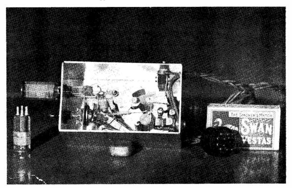
Inside the Grid Dip Oscillator — the valve mounting can be seen lower left, with the tuning condenser (Cl in circuit diagram) at the centre. The octal plug takes HT and LT supplies from one of the sockets seen on the Beginner's Power Pack on p.267 of the July issue.
