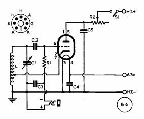
Fig. 1. Circuit of the Grid Dip Oscillator, for which full details Fig. 1. Circuit of the Grid Dip Oscillator, for which has defails for construction, calibration and uses are given in the article. The valve is a 9002 miniature triode, few pr. ts are called for (see table for values) and the circuit is of the simplest — yet it is safe to say that, when it comes to the building of trans-mitters, without a GDO you can hardly find your way about the bands.
