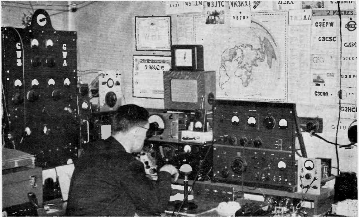
The neat outfit at GW3GWA, Wrexham, who is equipped for all bands from 3.5 to 144 mc. The main receiver is a BC-348 and to the immediate right of this in the photograph is the two-metre equipment, in rack form: Above, the 25w. transmitter and, below, a G2IQ-type converter; standing on the BC-348, to the right, is a CC converter. The beam for two metres is a 4-element Yagi and gear is in hand for Seventycems.
