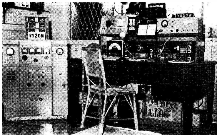
In the February issue we published a picture of Tan bin Hussain as an SWL; here is his station as VS2DW, a call actually held since 1952. Incidentally, he is the only native-born Malay in the world holding an amateur licence. As can be seen, he has a fine array of gear, including a modified BC-610E with a BC-221 as VFO, an HRO-7 receiver with Radiovision pre-selector and a 100 kc calibrator. Activity at present is almost exclusively DX-chasing on 80 metres, a most difficult band to operate in Malaya, and VS2DW remarks that he "spends more time tickling bug than gripping mike"
