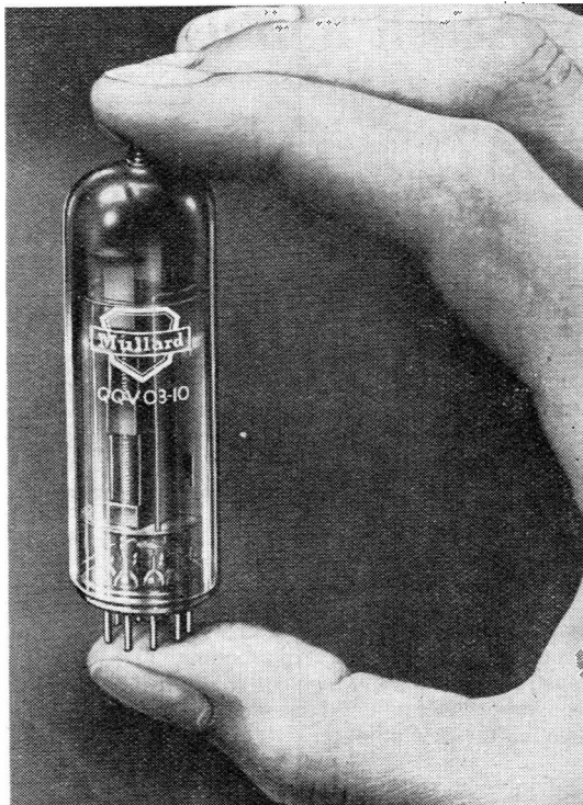
An interesting size comparison for the Mullard QVO3-10, which is a double RF tetrode with many applications in low-power and driver stages.
