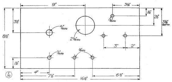
Fig. 2. Drilling detail for the front panel of the 14/21 mc switched two-band transmitter. This drawing should be carefully compared with the front panel view.
