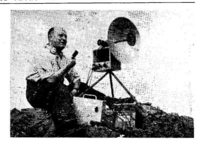
G8DD in action on 1250 mc at his /P site on Brown Clee Hill, near Ludlow, Worcs., on July 26 last, when he and G3QC/P were in QSO to raise the 1250 mc world record to 100 miles. Gear used was the same as at G3QC/P.
