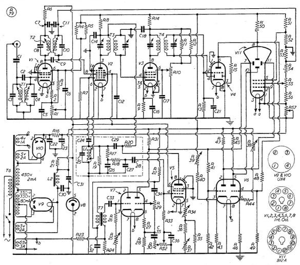
Fig. 5. Circuit complete of the panoramic adaptor unit ("panadaptor") described in the accompanying article. The frequency modulator section is enclosed in the dotted square, and all values are given in the table herewith. (Note: T3 is represented by the FM section).
