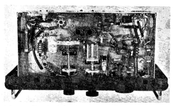
Layout under-chassis of the Two Band Table Topper, which gives ample RF output on 14 and 21 mc by switch control, with VFO drive.
