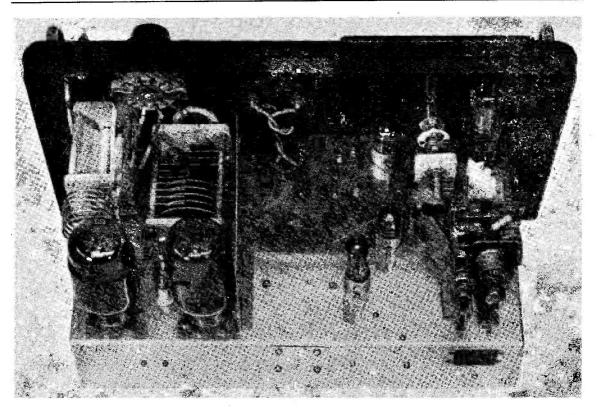
Rear chassis layout of the 14/21 mc band-switched transmitter, which runs Osram valves throughout with a pair of KT66's in the PA stage (left). This view shows many constructional details.
