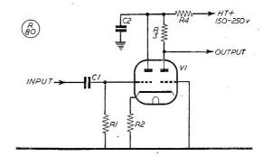
Fig. 6. Cathode coupled amplifier for the Panadaptor, values for which are given in the table.
