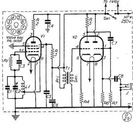
Fig. 1. Circuit of the all-band CW monitor suggested by G2NS.
