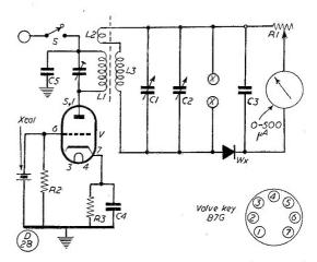
Circuit complete of the capacity meter suggested in this article. It can be calibrated by reference to a few good fixed condensers of known value. (Note: Trimmer across L1 should be marked C6).
