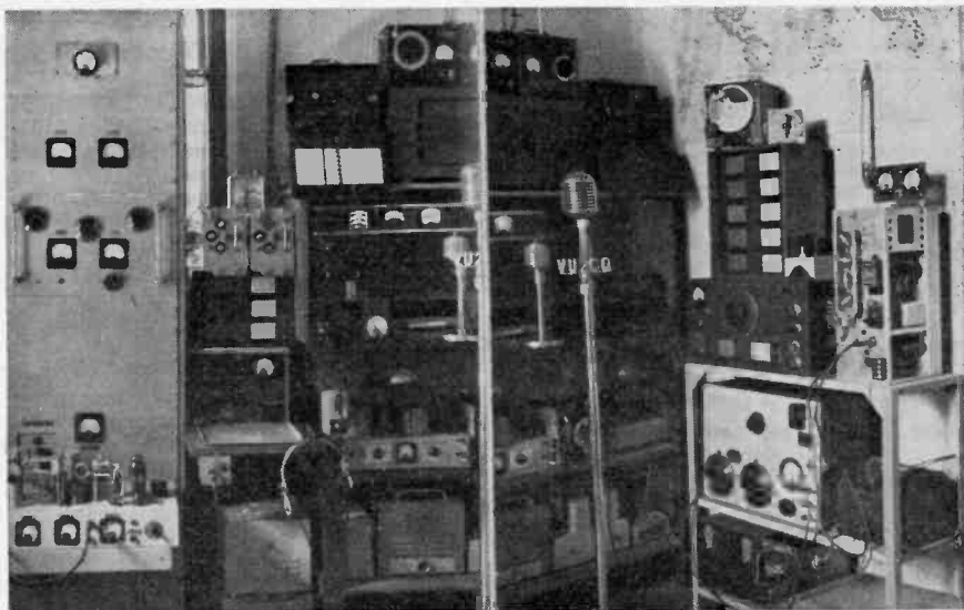
VU2CQ, Bombay, runs 100 watts to a pair of VT104's on 3.5, 7, 14 and 28 mc, Class-B modulated with a pair of 830B's, one aerial being a Sterba curtain. On 50, 56 and 144 mc, on which bands he is also active, VU2CQ has an 829 PA at 60 watts input. Receivers are AR88, HRO and ex-RAF 1337, 1338, with RF Units Type 26 and 27; he also has an SCR-522 converted for 288 mc. Other equipment includes a BC-221 and a wire recorder. VU2CQ has worked 148 countries on 'phone, and is a well-known DX signal.
