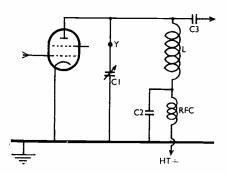
Fig. 3. Series-parallel suggested by G5UM. feed, the modification Fig. 3. Series-parallel feed, the modification suggested by G5UM. C1/L are effectively in parallel via C2, and the circuit tunes quite normally. One side of C1 can be earthed and the DC voltage across it removed by inserting an additional series condenser at Y. It is necessary to provide a good RF path from C1 through C2 to L, since the RF circulating current flows in this part of the circuit.
