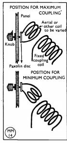
Fig. 5. R. A. Bernard's method of obtaining panel-controlled variable coupling. With extension rods, it could be applied to transmitter links.
