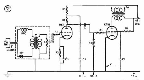
Fig. 2. Circuit of the modulator. A carbon microphone is shown, for which one stage of speech amplification (H63) is sufficient. This would not give enough gain with a crystal microphone, for which an additional stage (and some re-design) would be necessary. If self-bias is desired, a 3-watt resistor of 170 ohms, by-passed with 25 μF, can be inserted at the point "X" in the cathode lead of the KT66.
