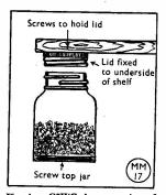
Fig. 4. G5WC has a series of screw-top jars for holding small parts. The lids are fixed by screws to the underside of a shelf and the jars screwed into the lids.
