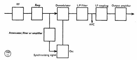
Fig. 1. Block schematic of the circuit arrangement. The attenuator-filter-amplifier element in the synchronising circuit may not be required in certain cases.
