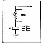
Fig. 6. Idea by P. H. Alderson. The 150,000-ohm resistor R limits the operating current for the relay RL.
