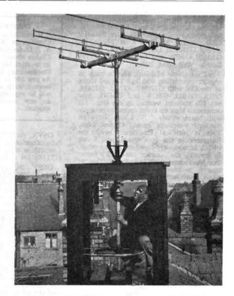
The 3-element rotary at G2IN. Southport, Lancs. The genera lconstruction of the beam and the method of rotating it can be followed from the photograph.
