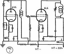
Fig. 1. The circuit of the original CO/PA, as described in the August issue. For anode-and-screen modulation of the 61.6, it is essential that Jack J be wired as shown. The modulator circuit is given in Fig. 2. Cathode control can be applied by breaking the cathode of the 61.6 and connecting the modulator output across the break.
