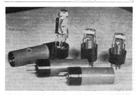
Showing the method of mounting the coils. Valve bases are used, with a paxolin tube to protect the coil. Note the hole in the tube for adjusting the padder.
