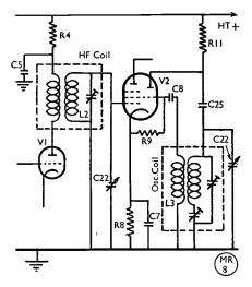
Fig. 2. Alterations to the circuitry around V1 and V2. Note the 100  $\mu\mu$ F condenser C25, inserted in the oscillator plate lead as a precaution against trimmer or padder condenser shorting on L3.
