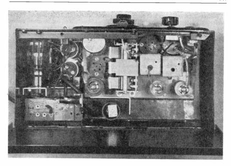
Looking into the receiver as modified. Rectifier valve on left, V1 in the first can at top with V2 in line below and the RF coll socket between them, aerial coil socket to the top right, and oscillator coil behind the screen along the lower edge. The space to the right of this screen could be used for an additional output stage.
