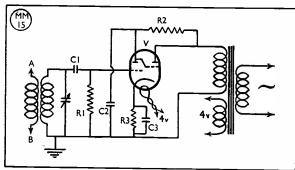
Fig. 3. Absorption wavemeter circuit suggested by P. E. Leventhall. A magic eye (Mullard TV4 or similar) is used to indicate resonance. Greatly improved accuracy is claimed for this arrangement.
