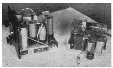
The receiver chassis and, on right, the power unit. The small extension to the chassis, as described in the text, can be seen with the meta screening for the oscillator.
