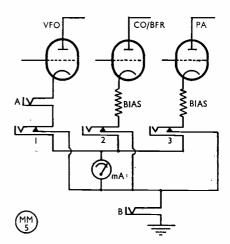
G3ADH's circuit for meter switching and keying. A shorting plug in jacks 1, 2 or 3 as required will produce plate current readings on the meter for the appropriate stage. Keying can be effected at either jacks A or B.
