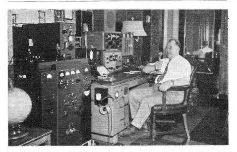
Clearly, VE3BKL of Merritton, Ontario, has practically everything! The transmitter is a BC-610 running just the half-kilowatt input, and receivers are a Super Pro and SX-28A.
