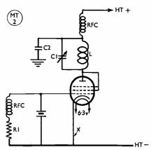
Fig. 1. Triode connected EF50, as tested by G5UM. This only worked satisfactorily when a 700-ohm bias resistor and by-pass condenser were connected at point X.
