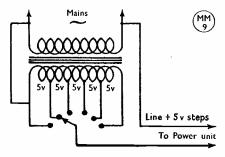
Fig. 1. Circuit of G2DYV'S arrangement. The boosting secondary can be a sufficient number of turns rough wound to give a total of 30 volts. The switch taps the required additional voltage to boost the mains.
