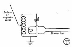
Fig. 2. Coupling the RF stage to an end-on or long wire aerial.
