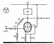
Fig. 3. Anode follower using cathode bias.
