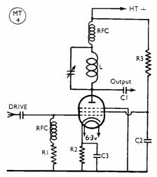
Fig. 3. A suitable frequency-multiplier circuit using the
