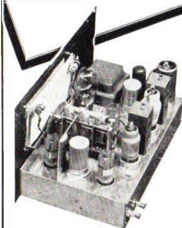
A high performance 6-valve A.C. Super-het covering 880 Kcs to 34 Mcs (9 to 345 metres) in 5 bands, having an EF 50 high-mu low noise RF stage.
