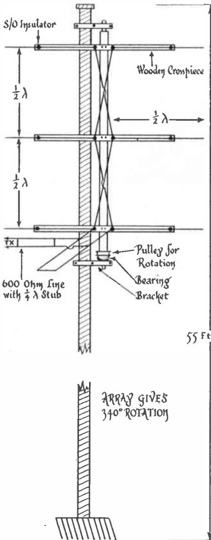
Diagram gives main details of the six- $\frac{1}{2}$ -wave-in-phase vertically stacked 58 mc aerial at G6CW (Nottingham). All elements are  $\frac{1}{2}$ -wave long, with  $\frac{1}{2}$ -wave separation, and fed through a 600-ohm line across a  $\frac{1}{4}$ -wave matching stub at the base of the array. G6CW credits this aerial with his recent successes on 5 metres.
