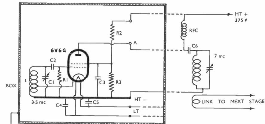
Fig. 1. Circuit of the VFO driver. Dotted lines indicate connections to external tank. Values are: L, 24 turns 16 SWG enamelled on standard plug-in former, with tap 8 turns from earthy end; C1, 160  $\mu\text{F}$ ; C2, 200  $\mu\text{F}$ ; C3, C4, C5, .01  $\mu\text{F}$ ; C6, .001  $\mu\text{F}$ ; R1, 100,000 ohms, 1 watt; R2, 50,000 ohms, 1 watt; R3, 20,000 ohms, 1 watt.
