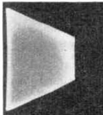
Fig. 28. Oscillogram of a signal with 38 per cent. modulation recorded without a time base.
