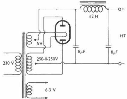
Fig. 3. A well-smoothed separate power supply is an essential for satisfactory operation of the VFO.
