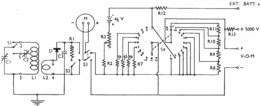
Fig. 1. Circuit of the Combined Instrument. S3 is the change-over switch, selecting either RF or DC measurements. By using an external battery, the resistance range can be multiplied up to ten times.
