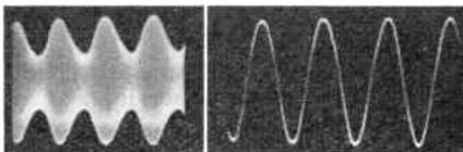
Fig. 30—Similar signal recorded with a time base. Fig. 31. Oscillogram taken from the diode stage of a receiver against a linear time base.
