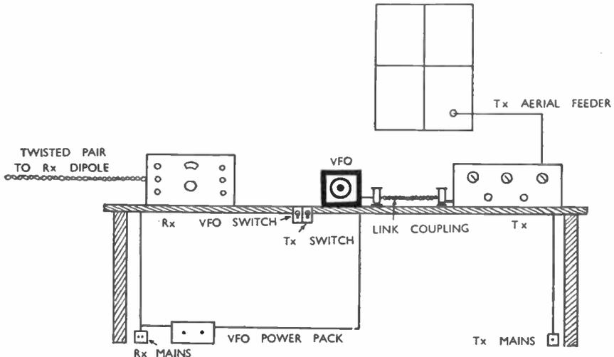
Fig. 4. Suggested internal station layout for using the VFO. Obviously, many variants of this arrangement are possible.
