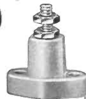
High-Voltage Microdenser Cat. No. 1094. Highly efficient. Soldered brass vanes. Constantly maintained capacity; very low minimum 3 mmfd. DL9 insulation. \frac{1}{4} " spindle extended for ganging. Peak flashover voltage 3,500 volts. Easy to gang—capacity matched within 1 per cent. 18 mmfd. 3/9
