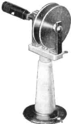
Neutralising Condenser. Cat. No. 1088. For HF circuits using low-capacity triodes. Maximum voltage 2000 volts D.C. Capacity variation 1-8 mmfd. Frequentite pillar insulator mounting, insulated adjusting knob. 6/6.
