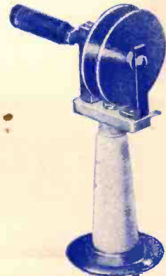
NEUTRALISING CONDENSER. Cat. No. 1088. For H.F. circuits using low-capacity triodes. Maximum voltage 2,000 volts D.C. Capacity variation 1-8 mmfd. Frequentite pillar insulator mounting, insulated adjusting knob. Price 6/6
