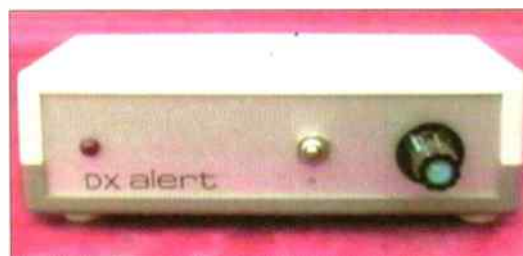
Fig. 5: A DXTV alarm which emits a warning tone when a signal is encountered.
