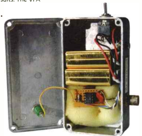
Batteries and amplifier board.
