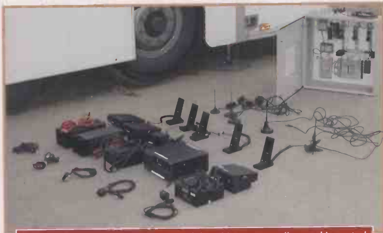
Counting back in. Some of the fixed mobiles with power supplies, used in control rooms. Plus a hybrid combiner and receiver distribution amplifier to allow three u.h.f. repeaters to share a single antenna.
