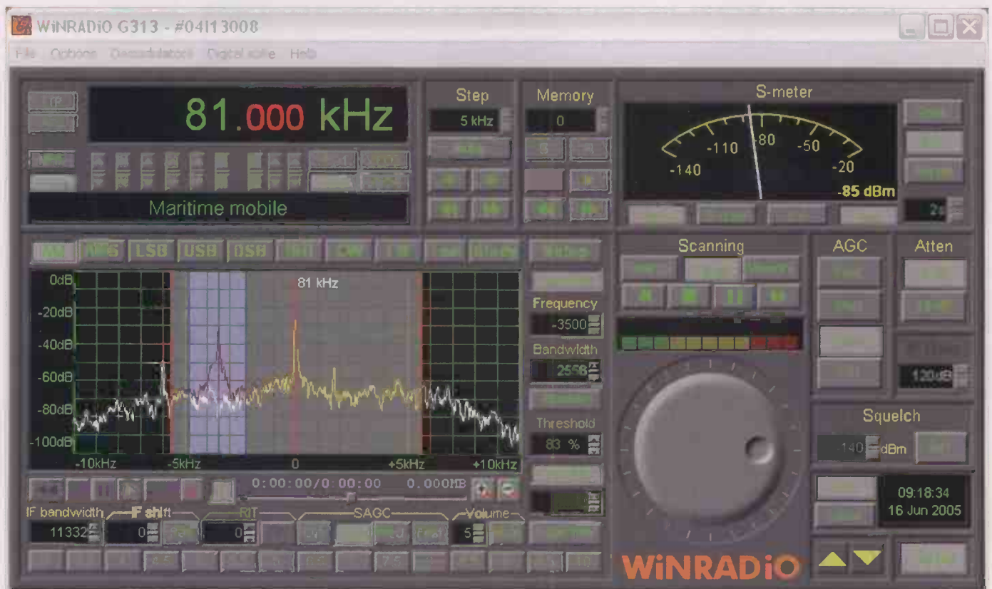
Fig.1: The bandscope now shows the plot before (dark red) and after (white) the i.f. notch filter.
