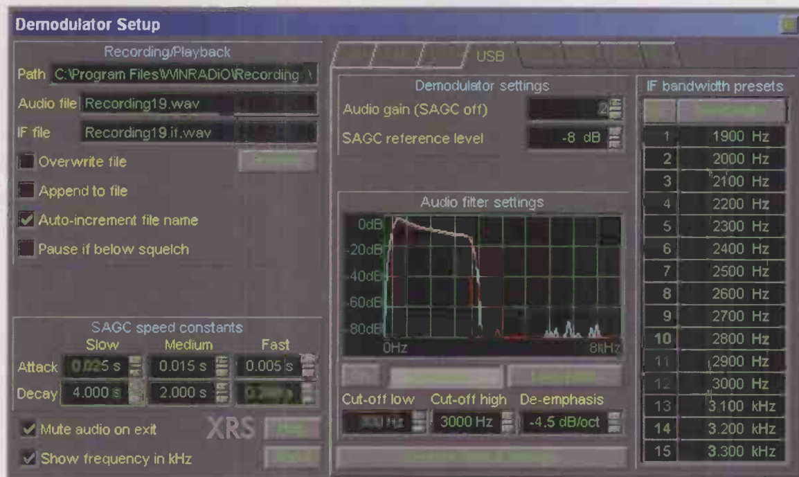
Fig. 2: The new audio filter appears in the Demodulator Set-up window. The red line shows the ideal filter pass-band, the blue line is the filter's actual response.
