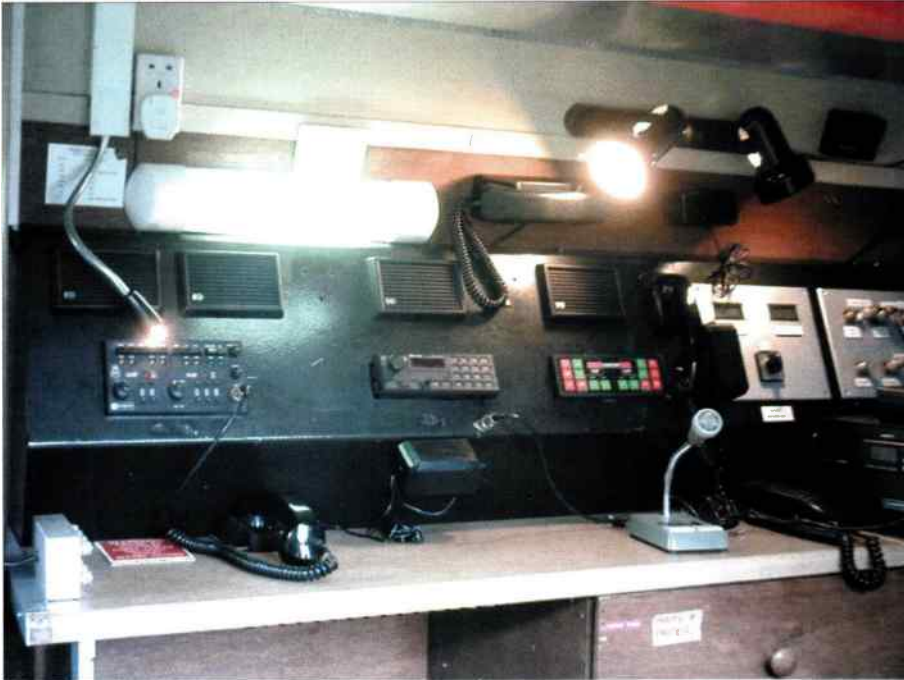
Interior shots of a recently decommissioned Police Mobile Control built into a Ford Transit van. The vehicle was from an 'East of England' force and you can see the Burndept v.h.f./u.h.f. repeater control and the Marconi RC690 sets together with speakers and other useful stuff including Anglepoise lamps that give a kind of 'X-Files' lighting effect.
