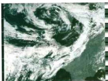
Fig. 4: NOAA-17 1113 22 August 2003 channel vis-2 showing successive passes of NOAA-17 and the image overlap.
