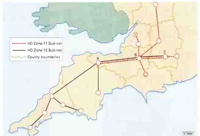
The two principal nets overlap between A and B and B and C. Between A and B parallel links are used because of path loss. Between B and C a single multiplex link is used.
