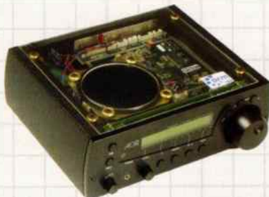
The modified AOR7030. The BBC DSP card can be seen on the right of the receiver, partly obscured by the loudspeaker. It's a perfect fit! (Picture courtesy BBC R&D).
