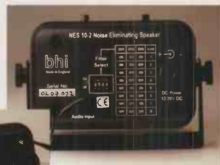
The DIP switch at the rear is used to select one of the eight preset levels.
