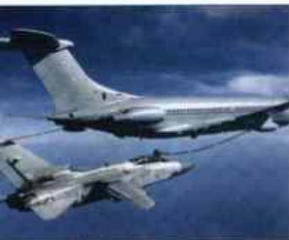
A close-up view of a Tornado F3 receiving fuel from a 10 Sqn VC-10 using the new underwing refuelling pods. (Crown Copyright).
