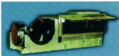
Fig. 1: The AVHRR instrument (courtesy NOAA).
