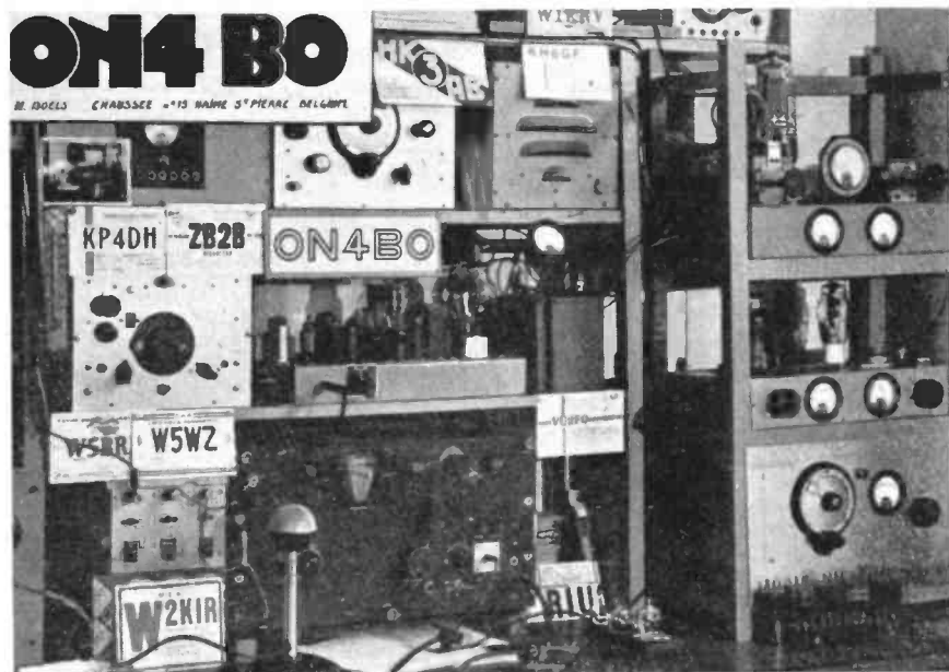
The fine QSL card sent by ON4BO. The Tx is a VFO-807 doubler-803 PA on 14 Mcs., with a rotary beam antenna. The Rx used is a BC 342
