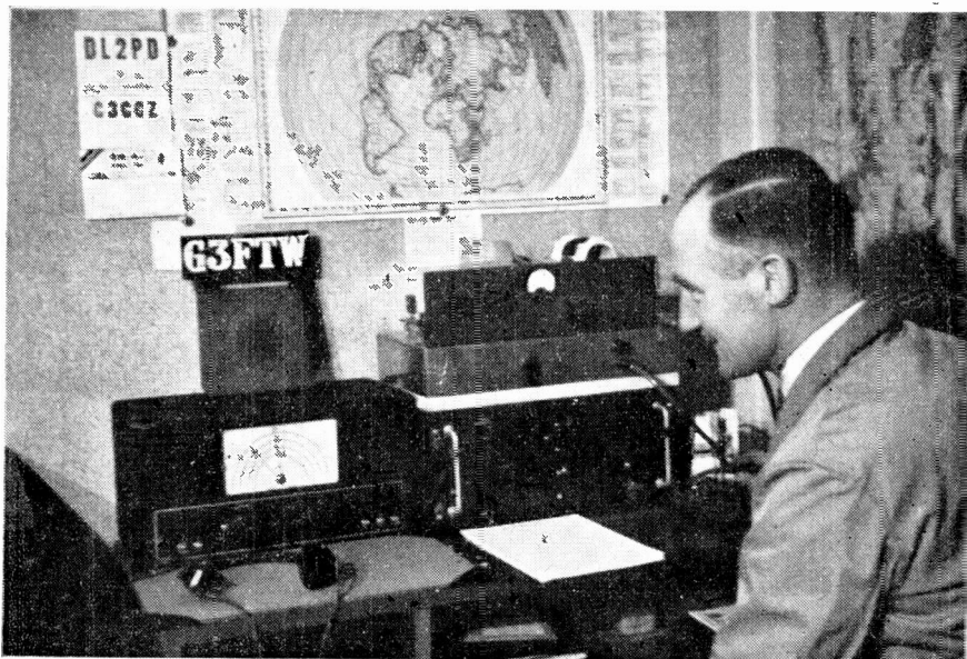
G3FTW of Dulwich, S.E.21., runs the "Transmitter for Beginners" described in the November-December, 1949, issues of our Short Wave Magazine. It is the unit top right of the S.640 receiver, and feeds into dipoles for 40- and 20-metre operation.
