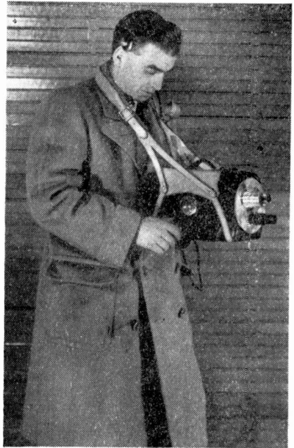
The Pye "candid camera" for roving TV reporters; it is both portable and compact.
