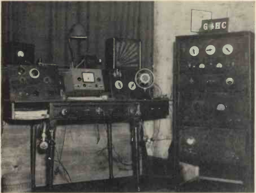
Station G4HC, Colchester, Essex. Though on a DC mains supply, AC power is obtained from a 400-watt rotary converter. The Tx is 6V6-807, the modulator uses P/P 6L6's in the output, the Rx is an HRO, and the aerial is as described in a pre-war issue of our Short Wave Magazine .
