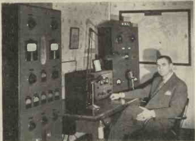
W3KXU, 415 Maple Avenue, Pittsburgh 18, Penna., U.S.A. runs 500 watts, VFO-controlled, on 14 and 28 mc, with a Hammarlund Super-Pro receiver and a 3-element rotary beam. This is actually his QSL card.
